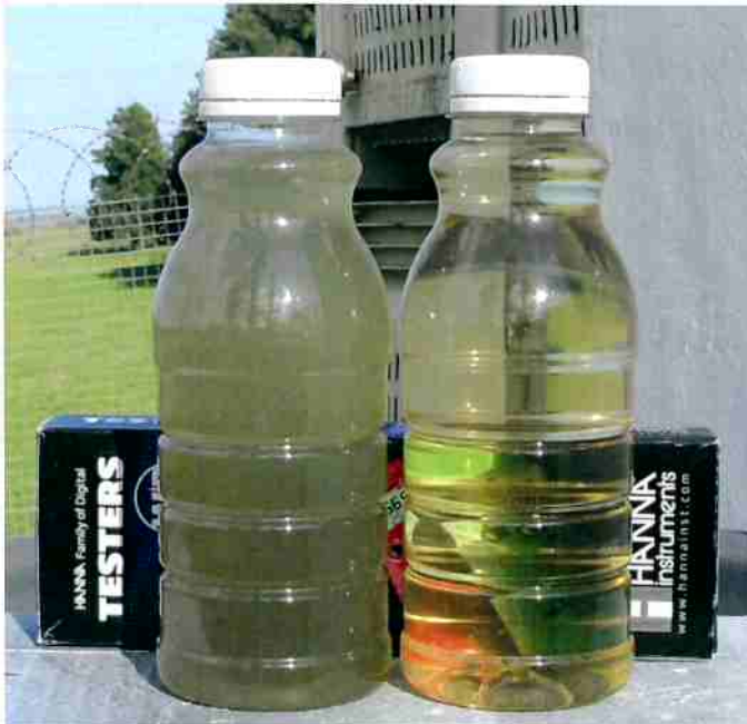
Samples. After inert solids interceptor on left and after The SOG Trickling Filter™ on the right.
